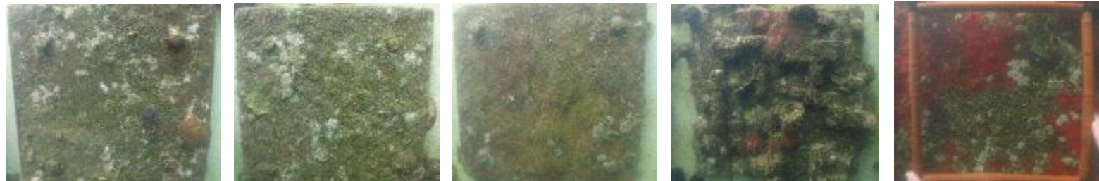
Tiles covered with marine growth 12 month post deployment
