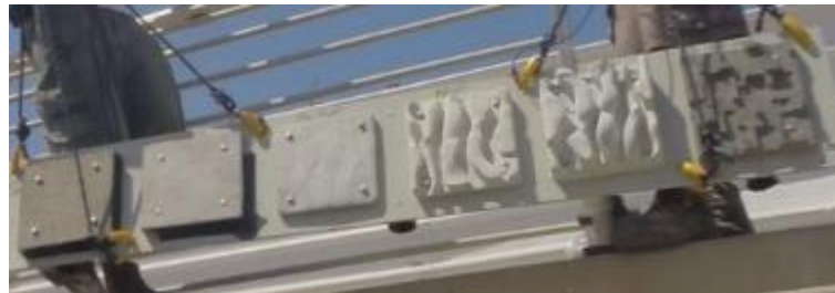
Tiles on the day of deployment, and existing seawall scraped as baseline control
